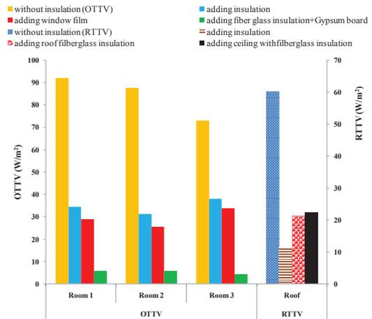
Figure 5. Average comparison of OTTV and RTTV before and after adding insulation materials.
