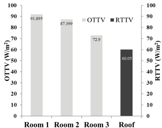
**Figure 2.** Results of OTTV and RTTV of the commercial building.
