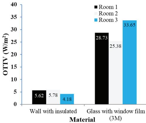
Figure 3. Averages of OTTV when adding insulation materials.
