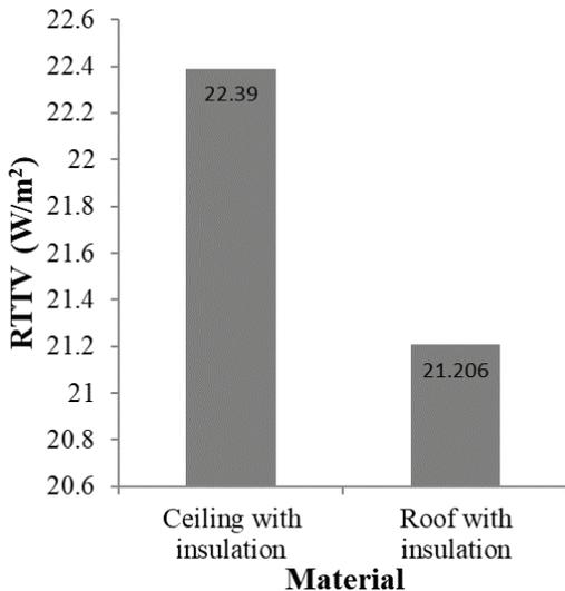
Figure 4. Averages of RTTV when adding insulation materials.
