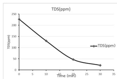
**Fig.14** TDS at different reaction times
