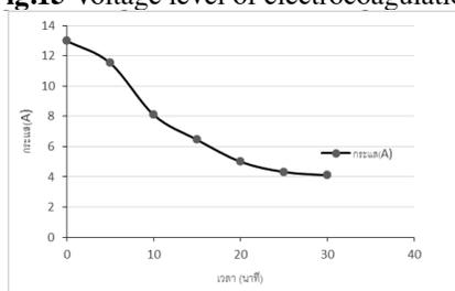
**Fig. 16** Current level of electrocoagulation
