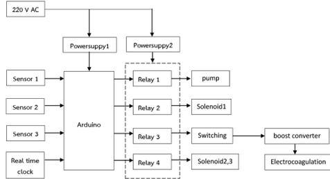
**Fig.7** microcontroller input-output diagram
