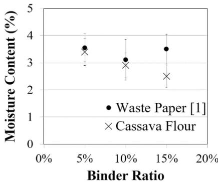
Fig. 3 Moisture content of sawdust briquette
