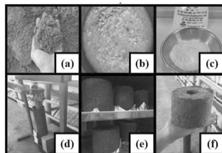
**Fig.1:** Raw material preparation and briquetting process
