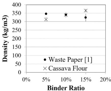
Fig. 4 Density of sawdust briquette
