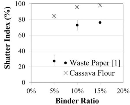
Fig. 5 Shatter index of sawdust briquette
